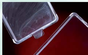
Blurry surface, caused by dust
